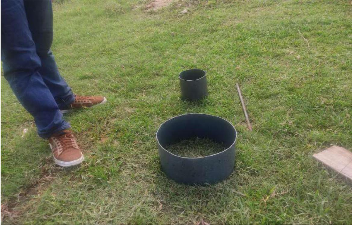
Soil infiltration test
